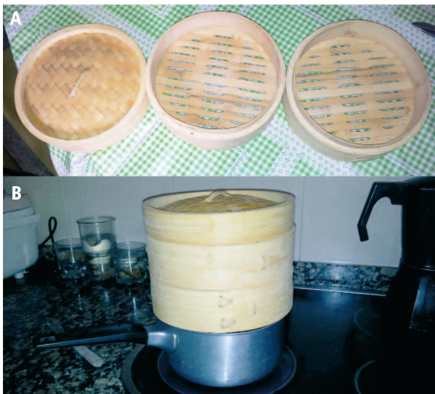
Fig. 3.- Photo of the steam column used in experiment 2. A) Storeys into which pumice samples were introduced. B) Experiment procedure. Boiling water is placed in the metallic container at the bottom.
