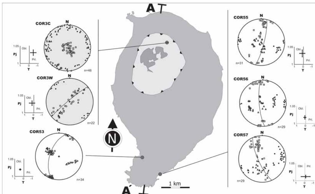
Fig. 4.- Stereoplots and anisotropy plots ( $P_j$  vs  $T$ ) for all the studied sites. Squares, triangles and circles, in the stereoplots, indicate  $K_1$ ,  $K_2$  and  $K_3$  directions respectively. The great circles represent the mean trend of the sampled dikes on each site.
