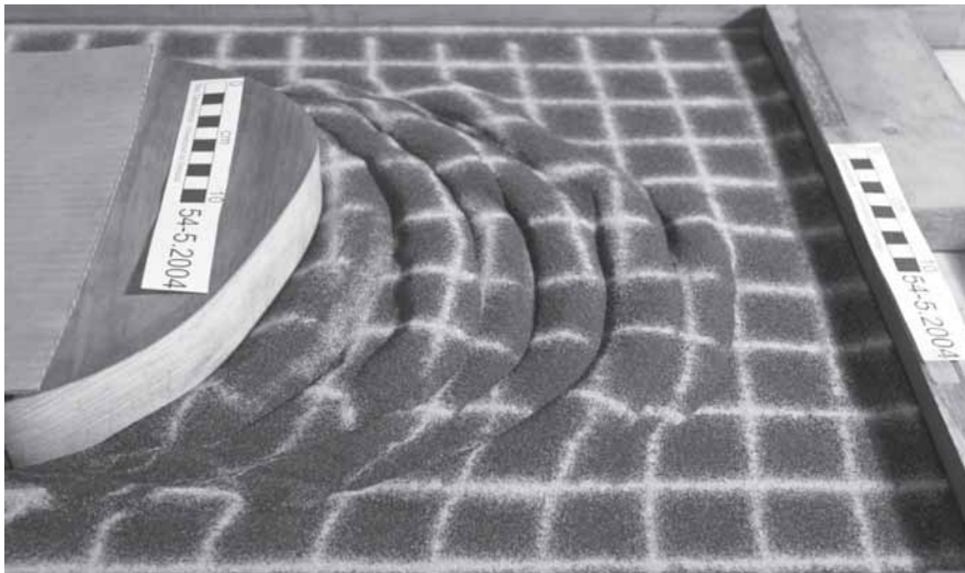
Fig. 4.- Oblique view of the final stage of the model composed by sand sieved over silicone.
