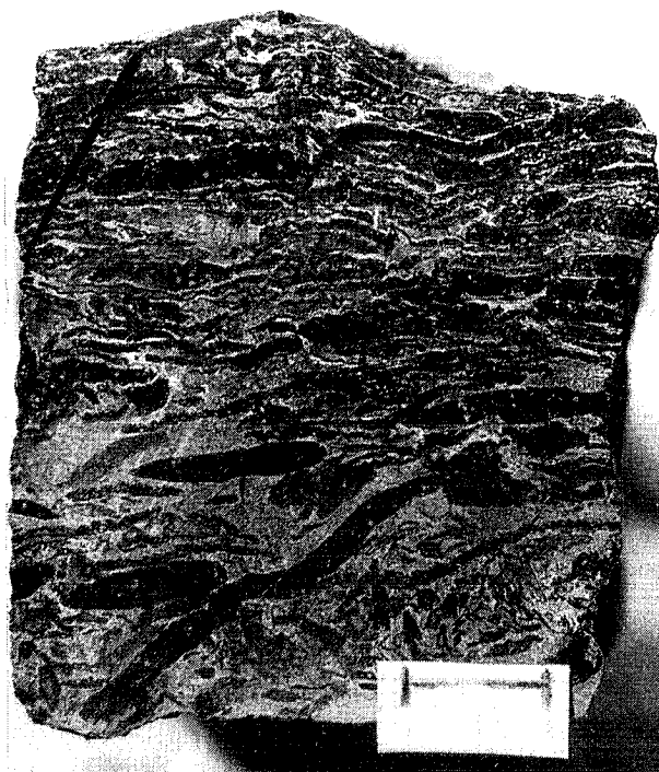
Fig. 4.-Ald. 1 Sample; Conglomerate with flattened phosphate pebbles (black) interpreted as gravel-lag contourite. Aldeavieja de Tormes. Scale bar = 1cm.
